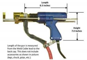
The TWE17000 is approximately 8.5" long from the weld cable to the back cap, and approximately 7" long from the top of the stud gun to the bottom of the handle. The overall weight of the stud gun is approximately 15 pounds ( with 8.5 feet of 4/0 weld cable and 8 feet of control cable (This also includes all connectors, legs, and foot piece.).
