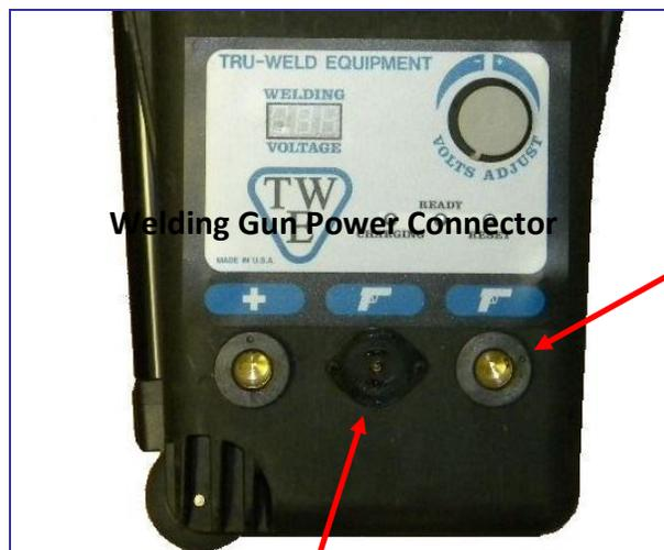
Welding Gun Control Cable Connector
