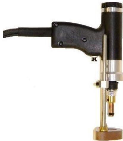
When removing the stud gun from the welded stud, always lift the stud gun vertically from the welded stud in order to maintain the proper tension of the collet. Spreading the collet when lifting the stud gun from the welded stud will shorten the life of the collet and will eventually create an undesirable weld.
